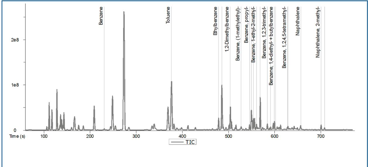
Figure 5. A chromatogram of 93-octane commercial gasoline is shown with peak markers automatically placed for the 23 calibrated analytes.
